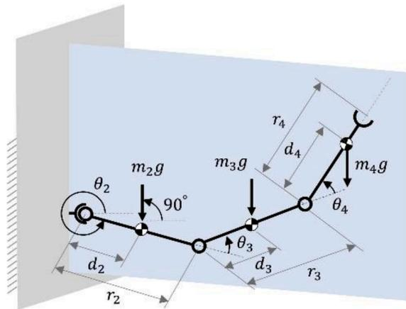
Fig. 3. An example planar articulated 4-link manipulator.
