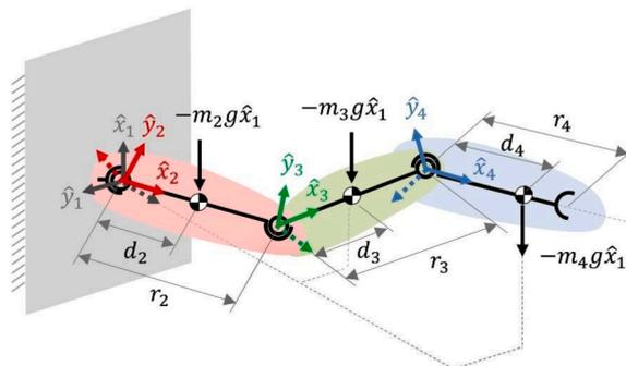
Fig. 5. Example of a four-link spatial articulated manipulator with spherical joints.
