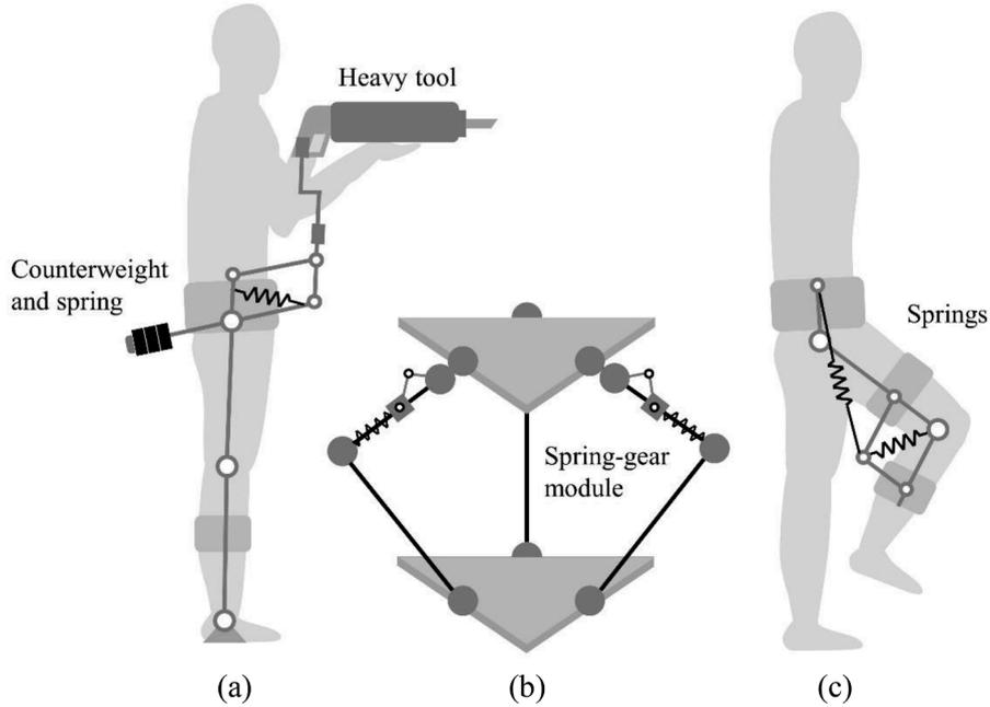
Fig. 2. Applications of gravity compensation technology: (a) industrial exoskeleton [23]; (b) spatial parallel mechanisms with spring-gear modules [14]; (c) spring balanced lower-limb exoskeleton [16].
