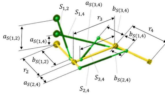
Fig. 14. A four-link spatial manipulator with springs  $S_{1,2}$ ,  $S_{1,4}$ ,  $S_{2,4}$  and  $S_{3,4}$ .
