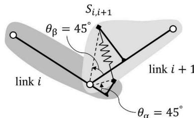
Fig. 12. Example of a mono-articulated spring attachment to a planar manipulator.
