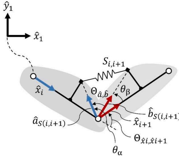
Fig. 11. Mono-articulated spring attached to a planar manipulator.
