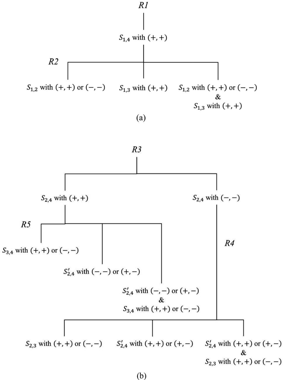
Fig. 13. The choices of spring installation for a 4-link spatial articulated manipulator.
