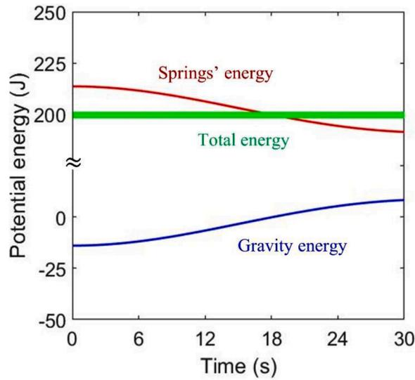
Fig. 16. Energy of the example manipulator during the simulated trajectory.
