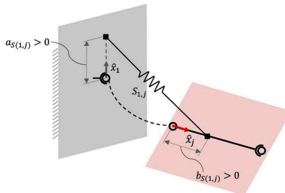
Fig. 9. Attachment of a ground-connected spring with  $(a_{S(1,j)}, b_{S(1,j)}) = (+, +)$ .
