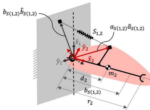
Fig. 8. Two-link spatial manipulator with spring  $S_{1,2}$ .
