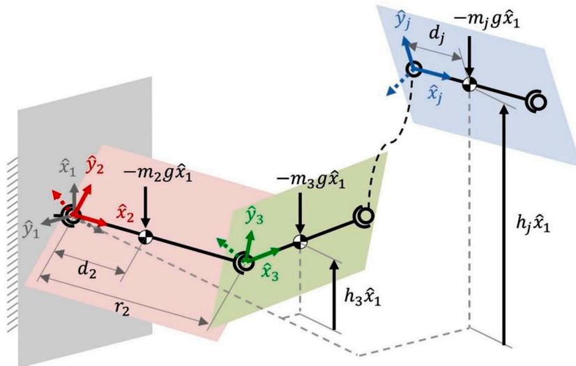
Fig. 4. Modeling of a general spatial articulated manipulator with spherical joints.
