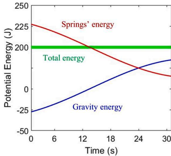
Fig. 17. Energy of the example manipulator during the planar trajectory.
