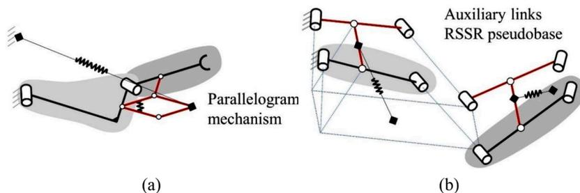
**Fig. 1.** Gravity balance of spatial articulated manipulators: (a) auxiliary parallelogram mechanism [11] and (b) pseudo-base formed by the RSSR auxiliary mechanism [12].
