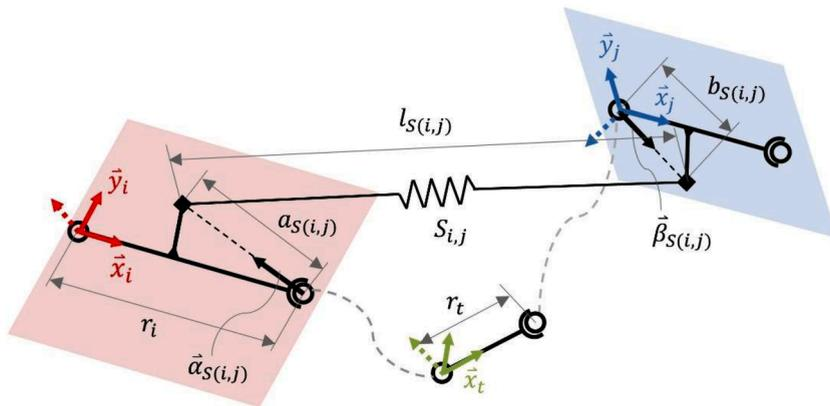
Fig. 6. Tension spring attached to a spatial articulated manipulator.
