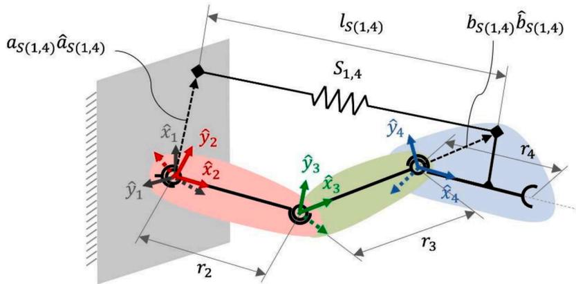
Fig. 7. Example spring attached between the ground link and the fourth link.
