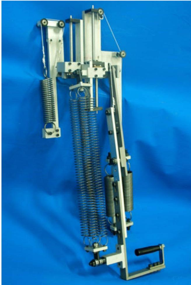
Fig. 6. The perspective view of the prototype of upper limb exoskeleton.
